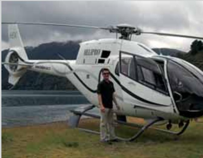
Fenestron tail rotor, which significantly reduces noise emissions.
